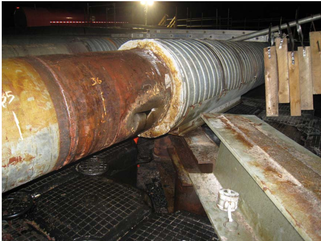
Photo showing the puncture in the BPXA DS 16 Flowline D and the wooden blocks to prevent the flowline from shifting. (10/17/07 Photo courtesy BPXA)
